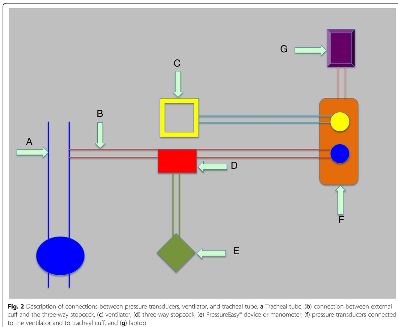
**Fig. 2** Description of connections between pressure transducers, ventilator, and tracheal tube. **a** Tracheal tube, **(b)** connection between external cuff and the three-way stopcock, **(c)** ventilator, **(d)** three-way stopcock, **(e)** PressureEasy® device or manometer, **(f)** pressure transducers connected to the ventilator and to tracheal cuff, and **(g)** laptop
